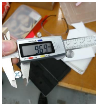
Using a Vernier calliper to measure the diameter of the cross dowel, and hence the size of hole needed to be drilled
