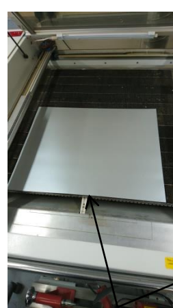
Laser Cutting the scale model from dxf to thin card into two sections (Seat and Shell).
