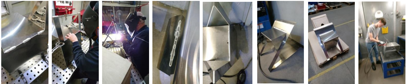
Above displays the welding process, the first picture tacking, the next two of a professional welding the product, the complete welds, the resultant shape of the shell, and myself blending the weld.
