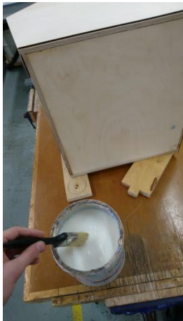
Applying the water based protective varnish.
