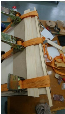
The above shows the flexi-ply was formed around the top curve.
