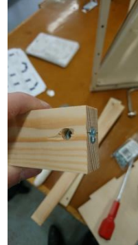
The fitting, secured into the tensioning piece
