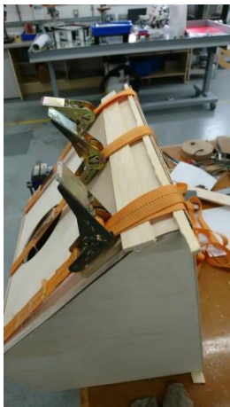
The above shows the flexi-ply was formed around the top curve.
