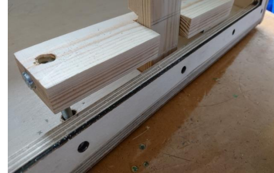
The tensioner installed before the strings were added
